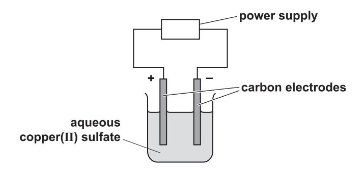
Oxygen gas forms at the positive electrode (anode).
